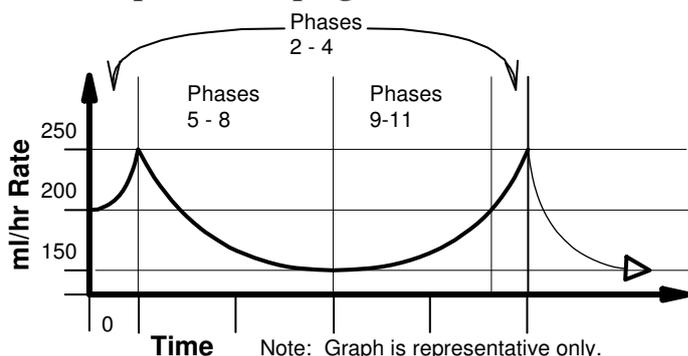
Continuously ramp up and down the pumping rate. Starting at 200 ml/hr, the pumping rate will increment to 250 ml/hr in 1.0 ml/hr steps after every 0.1 ml has been dispensed. Then the pumping rate will decrement to 150 ml/hr in 1.0 ml/hr steps after every 0.1 ml has been dispensed. Finally, the pumping rate is incremented back to 200 ml/hr in 1.0 ml/hr steps after every 0.1 ml has been dispensed, then the process is repeated.
