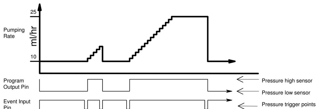
This example demonstrates a Pumping Program whose control depends on an external sensor. Assuming a pressure sensor that is configured to detect a high pressure point and a low pressure point, the Pumping Program individually selects whether it will react to the high or low pressure point.
