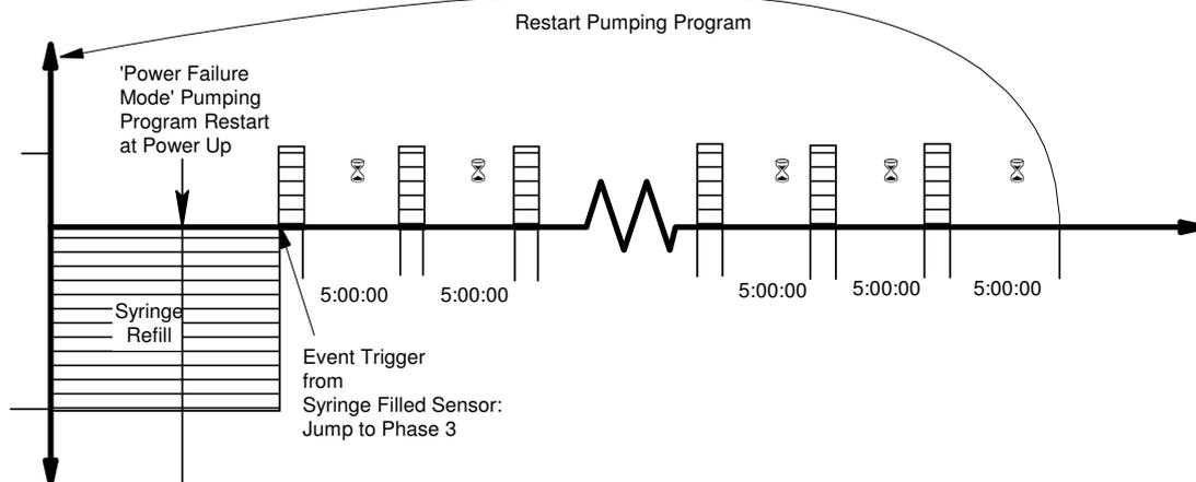
The following is an automated dispensing Program for a NE-1600/NE-1800 syringe pump equipped with a 'Syringe Filled Sensor' (part #ADPT-1) attached to the TTL I/O connector, and a valve system to refill the syringe from a reservoir. It is also assumed that the 'Power Failure' mode is enabled.
