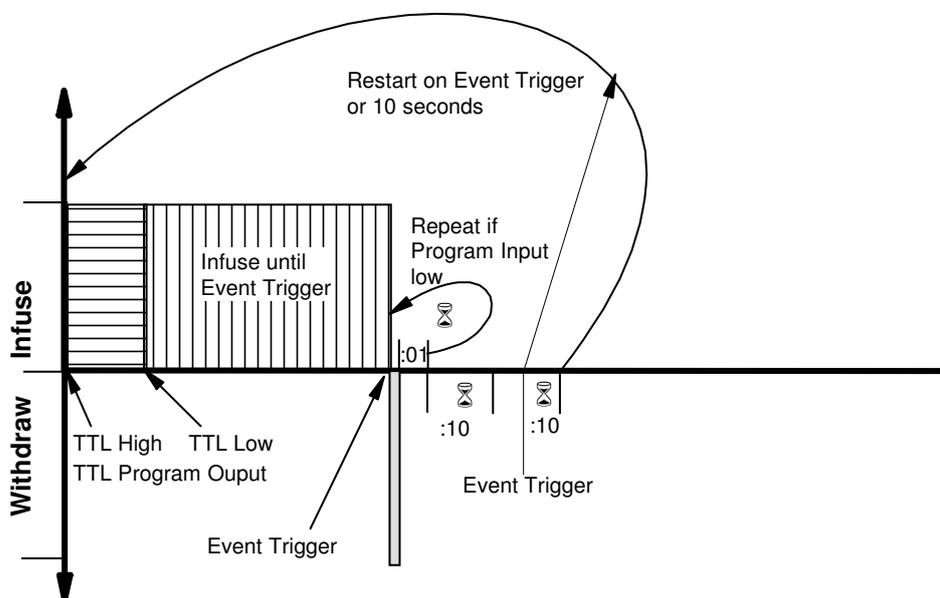
This example demonstrates a complex interaction with external equipment, such as synchronizing with another syringe pump. The Program includes a variety of interactions with external equipment, which demonstrates the various control possibilities of the NE-1600/NE-1800.
