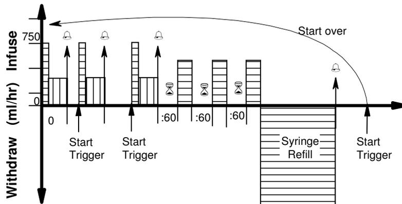
A more complex dispensing example, this Program contains different pumping requirements, including dispenses with multiple pumping rates. The first set of 3 dispenses drops down to a lower pumping rate during the dispense. When each dispense is completed, the buzzer beeps to alert the operator, then the pump waits for a start trigger before starting the next dispense.
